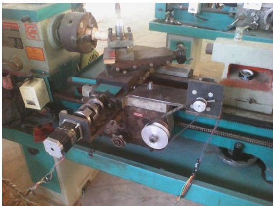
Figure 8 Actual Final Assembly on Lathe Machine
